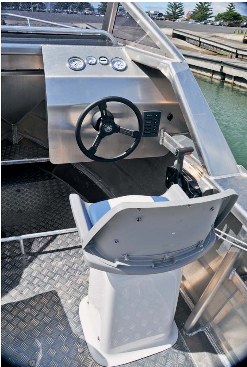
Helm seats are upholstered plastic-bucket type with fold-down backs.
