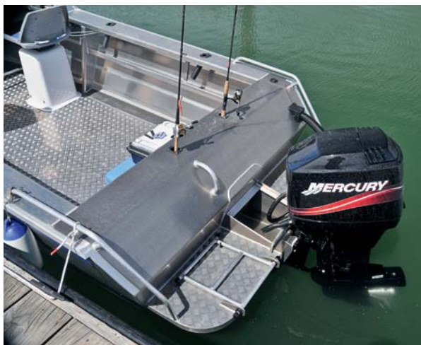
Grab rails, ladder and boarding platform aid divers.
