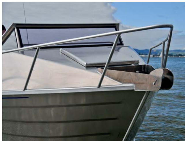
A large forward hatch gives comfortable access to work the anchor.
