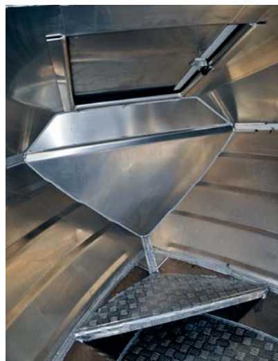
A platform is fitted in the bow as an aid to pulling the pick.
