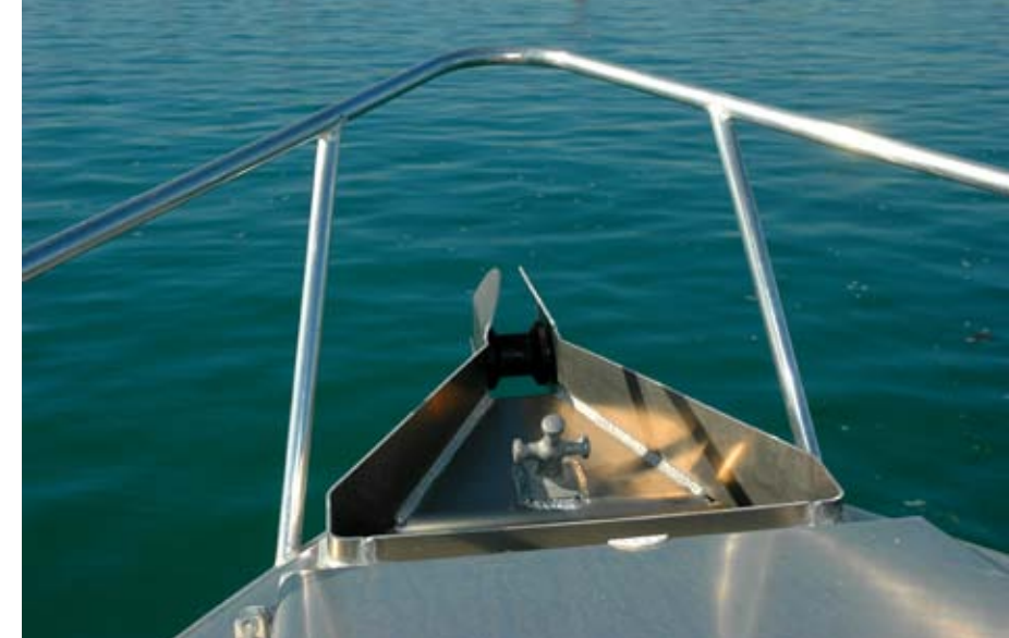
The open anchor locker can be fitted with an auto winch.
