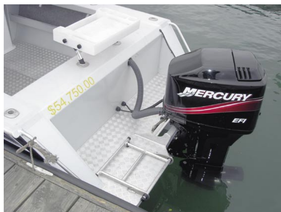
A boarding ladder, grab rail and platform are a boon for divers.
