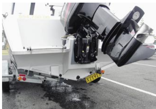
Separate plates allow fitting of trim tabs and transducers without drilling into the hull.
