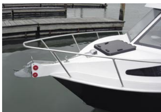
A permanently mounted anchor and electric capstan make light work of anchoring.
