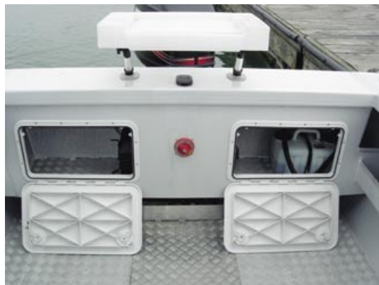
Front-opening hatches access the transom locker.
