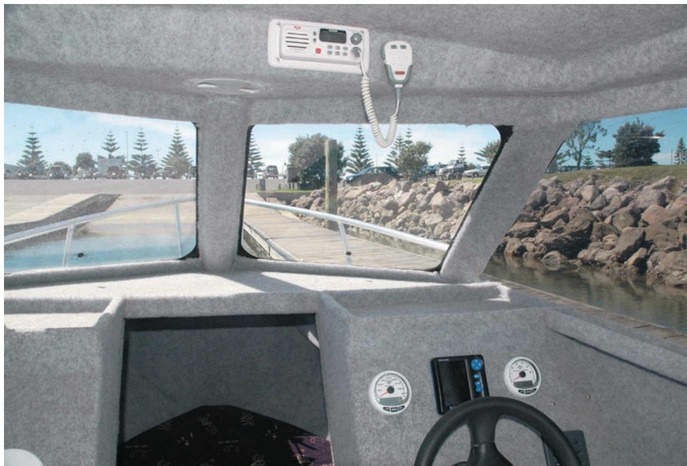
Basic instrumentation, switching and a sounder are flush-mounted at the helm; a VHF is set overhead.
