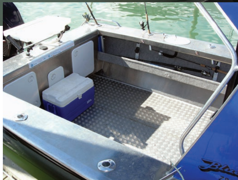
The saltwater basin set in the gunwale top is useful for washing hands while fishing.
