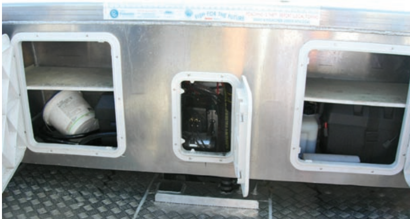
The customised transom lockers hold the batteries and provide further stowage space.
