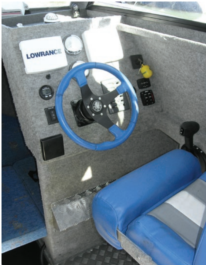
The leading edge of the helm seat can roll back to make more space for a standing helmsman, providing a backrest at the same time.
